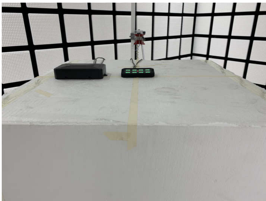
Radiated spurious emission Test Setup-2(Above 1GHz)
