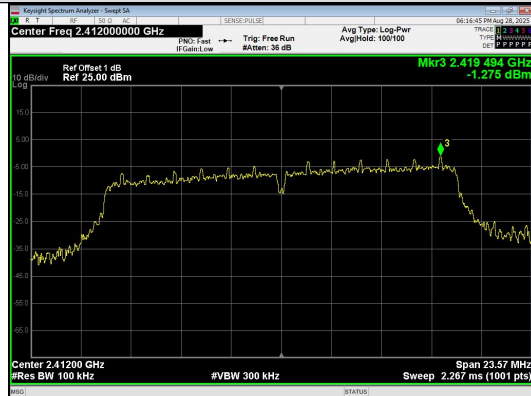
In-Band Reference Level IEEE 802.11g_Channel 1_20MHz_Antenna 0
