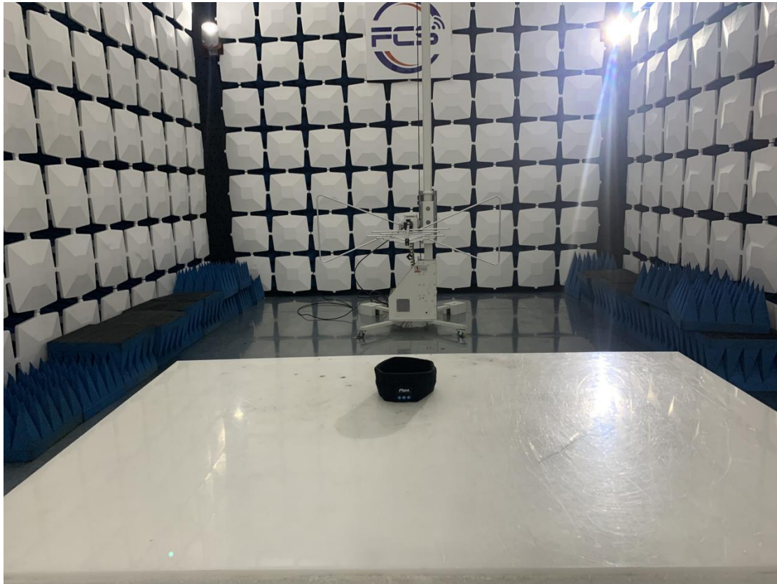
Above 1GHz for radiated emission test setup
