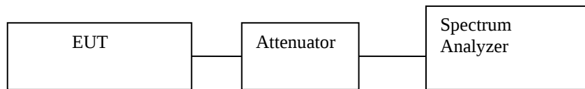
Figure 2. Block Diagram, Occupied Bandwidth Test Setup
