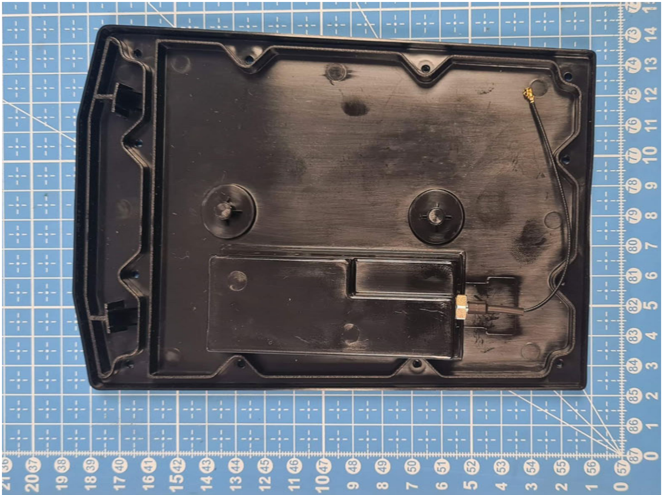
Figure 6 - Rear of the Enclosure - \mu FL to SMA Connector
