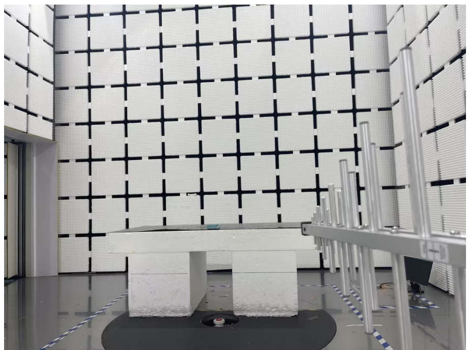
Radiation Emission Test Setup (30MHz to 1GHz)
