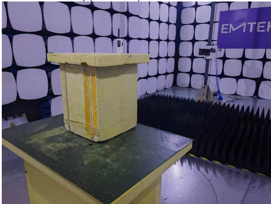
Spurious Emission Test Setup (Above 1GHz)
