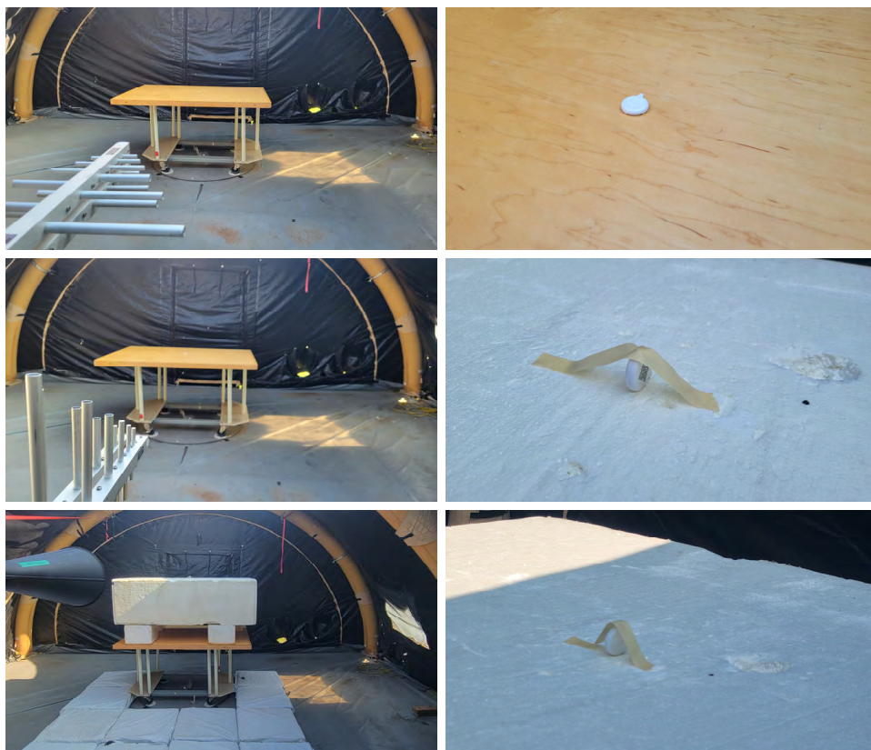
Figure 4: Radiated Emissions Test Setup Photograph(s).
