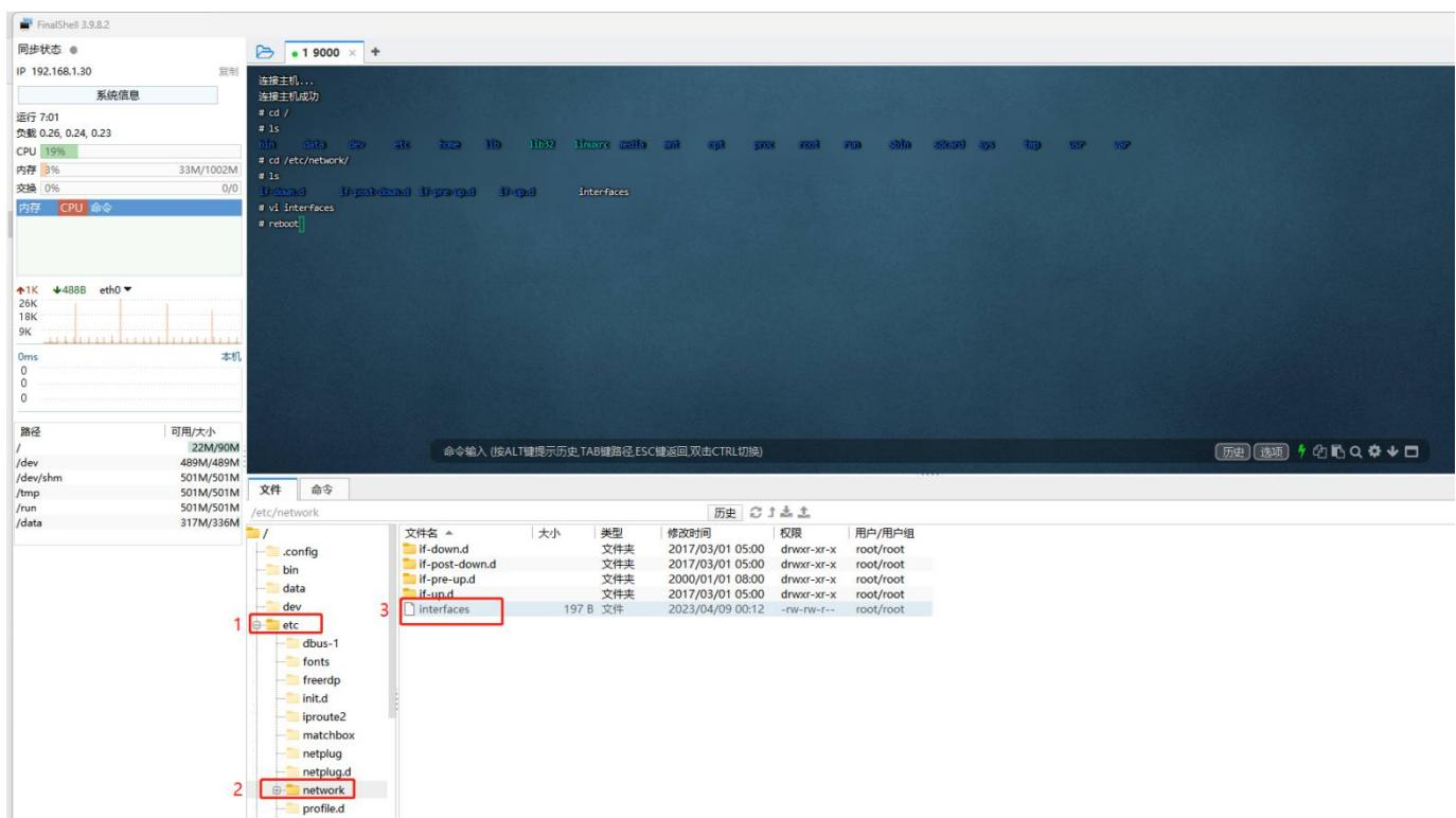
**4.2** Double-click on the file “Interfaces”, and change the IP address and gateway address of “address” and “gateway” in the file to the values required by the project as shown in the figure below.
