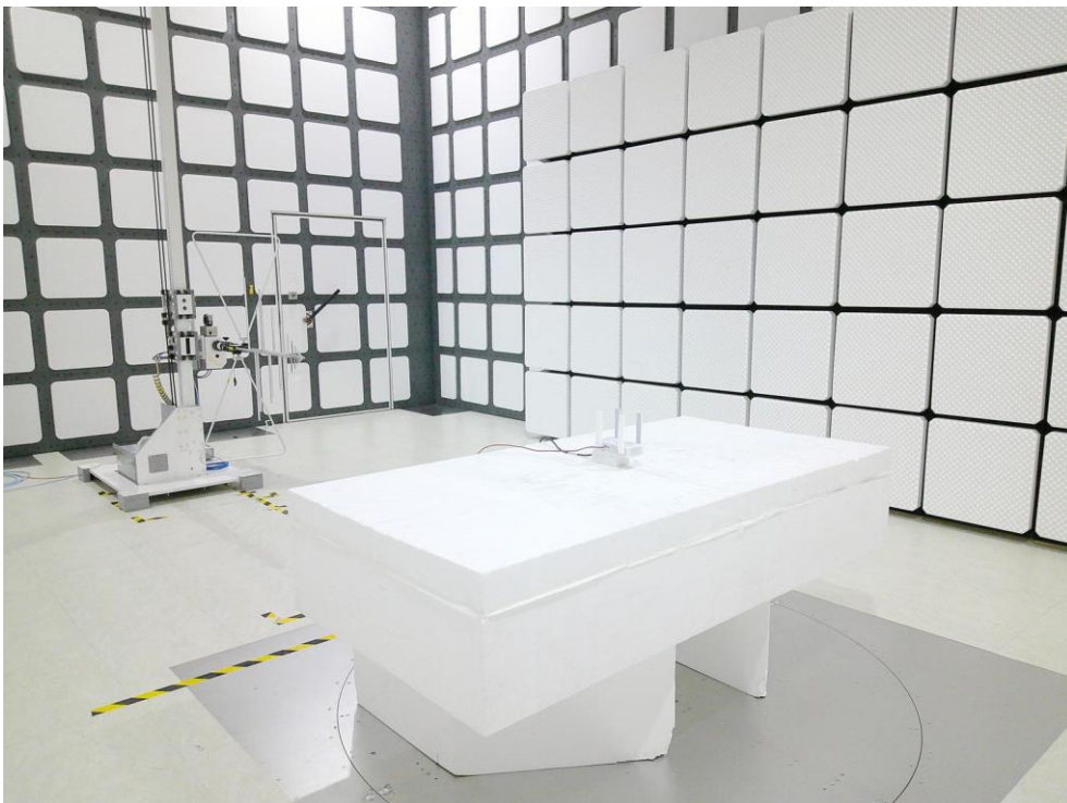
Description: Radiated Emission Test Setup for 30MHz~1GHz
