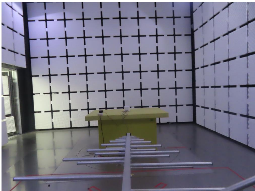
**Radiated Emissions Test Photos****Band edge**
