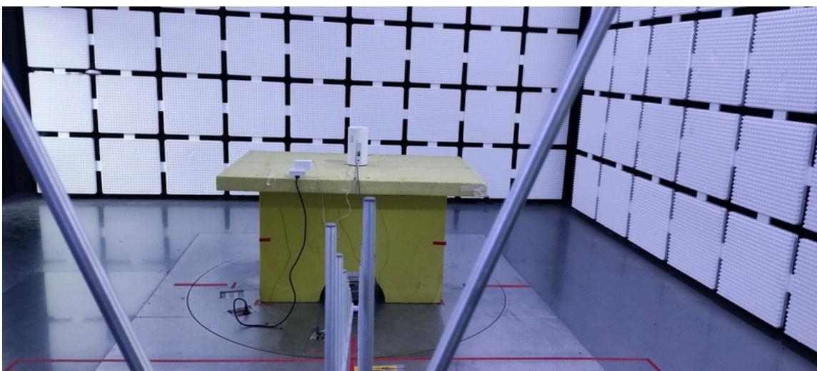
**Radiated Emissions Test Photos****Above 1 GHz\_Band edge & Harmonic(1 GHz to 18 GHz)**
