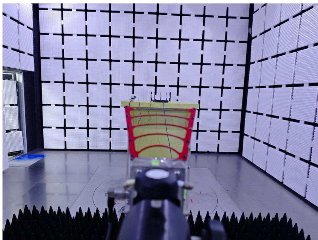
**Radiated Emissions Test Photos****Above 1 GHz\_Harmonic(18 GHz to 26.5 GHz)**
