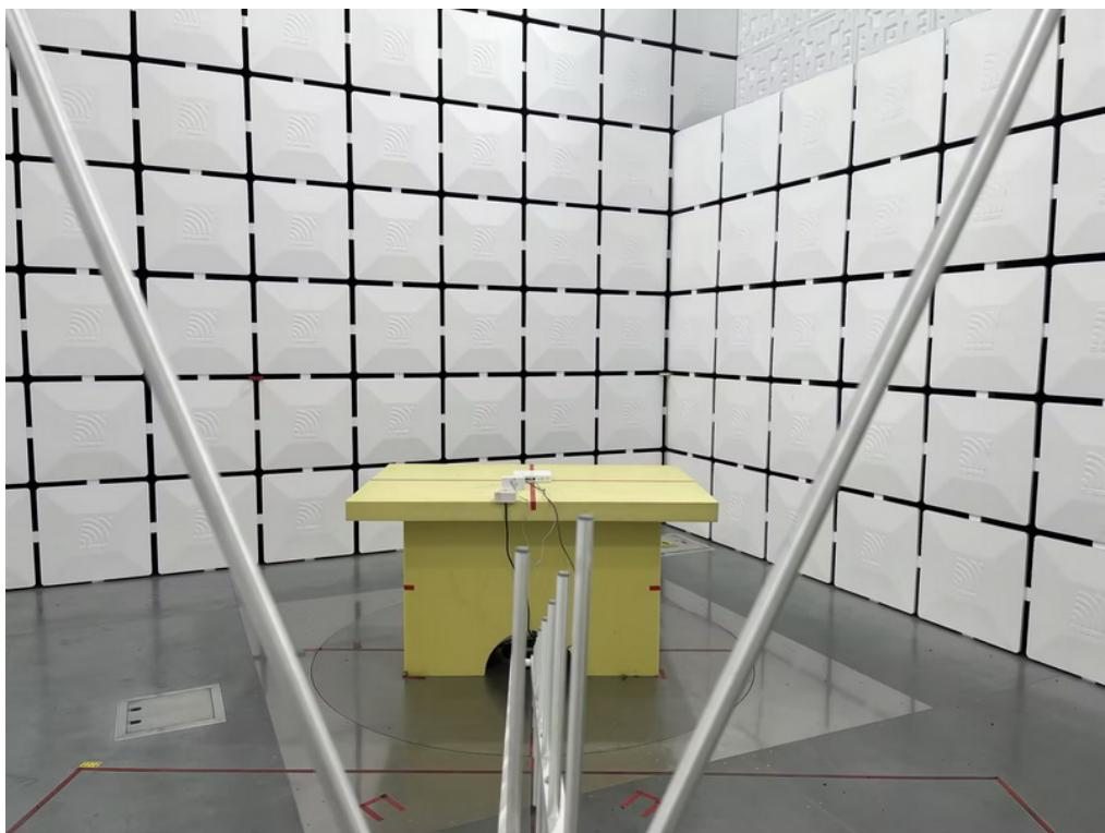
**Radiated Emissions Test Photos****Band edges & Harmonic 1 GHz-18 GHz**
