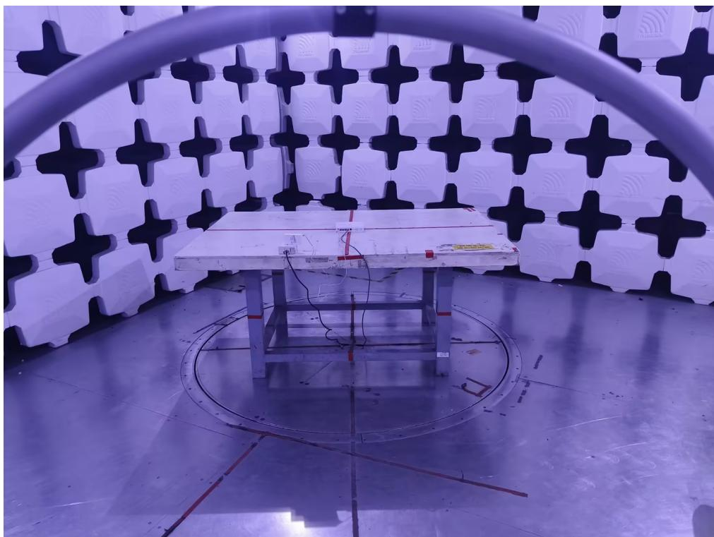
**Radiated Emissions Test Photos****30 MHz to 1 GHz**
