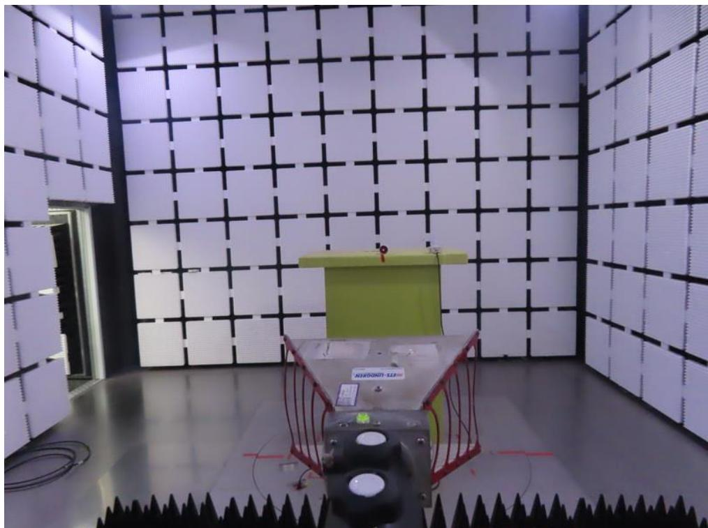
**Radiated Emissions Test Photos****Harmonic(18 GHz to 26.5 GHz)**
