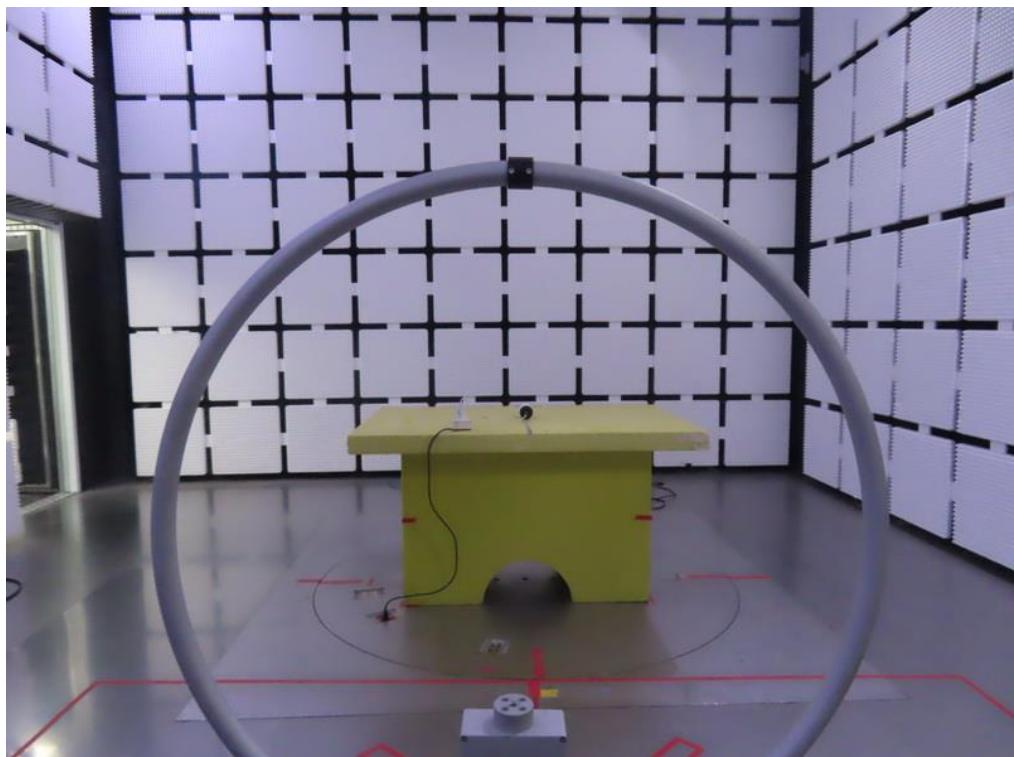
**Radiated Emissions Test Photos****30 MHz to 1 GHz**
