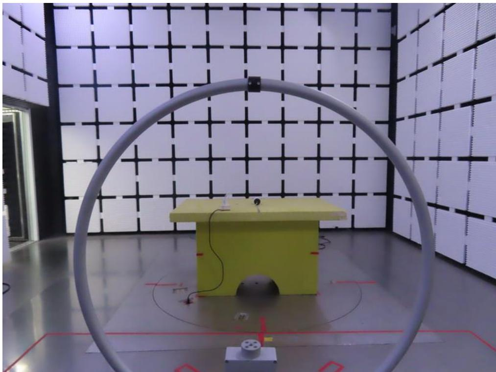
**Radiated Emissions Test Photos****30 MHz to 1 GHz**
