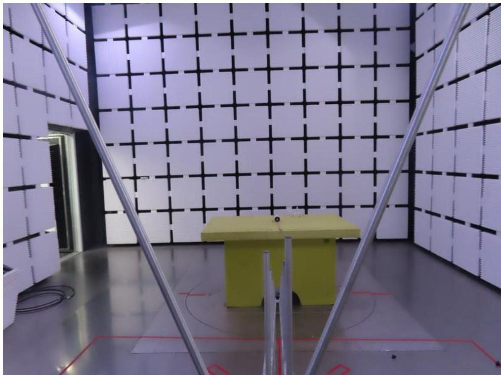
**Radiated Emissions Test Photos****Band edge & Harmonic(1 GHz to 18 GHz)**
