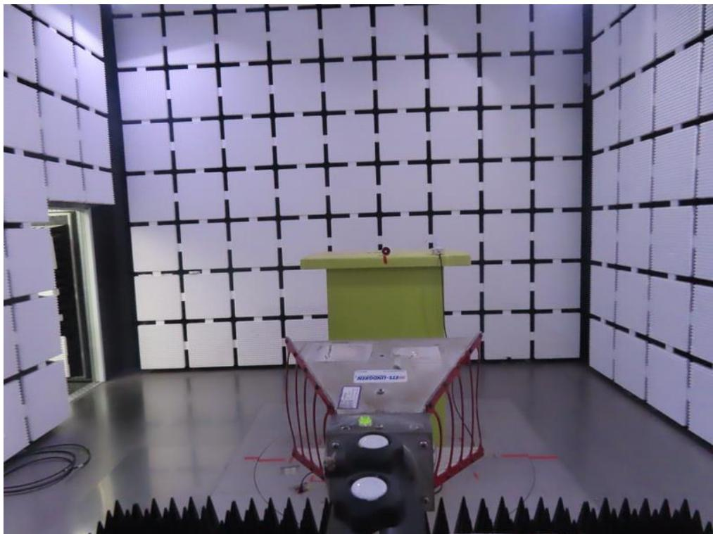
**Radiated Emissions Test Photos****Harmonic(18 GHz to 26.5 GHz)**
