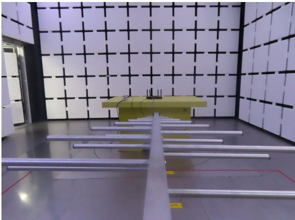
**Radiated Emissions Test Photos****Above 1 GHz**
