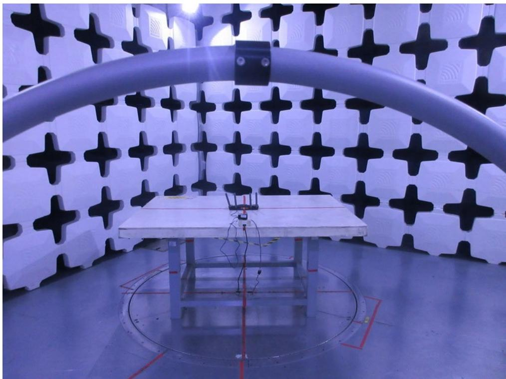
**Radiated Emissions Test Photos****30 MHz to 1 GHz**
