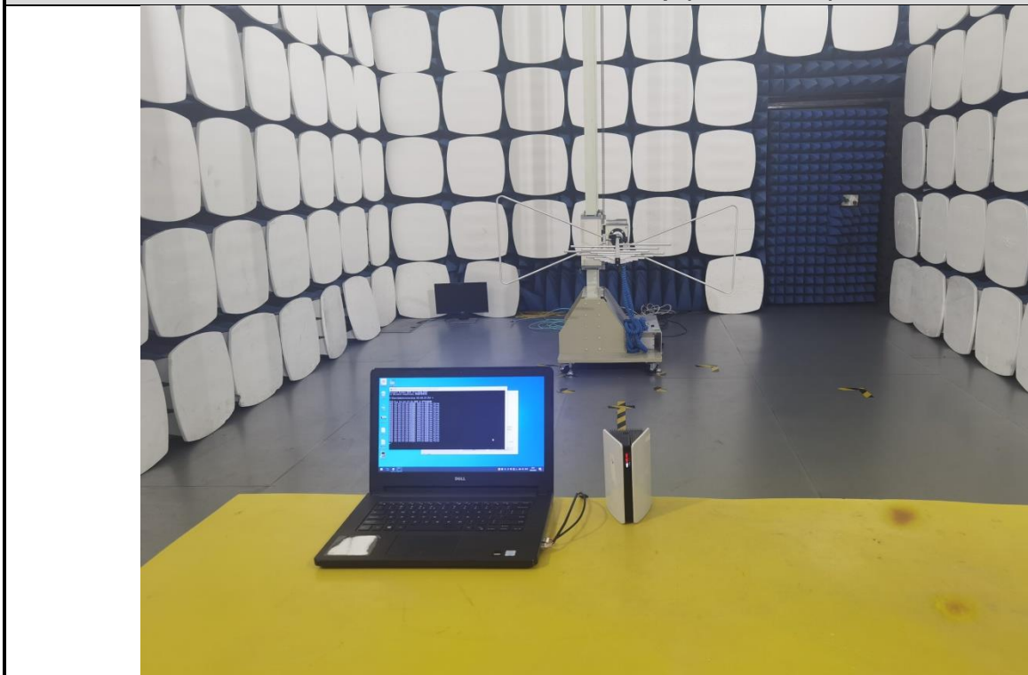
Radiated emission Test Setup (Below 1GHz)
