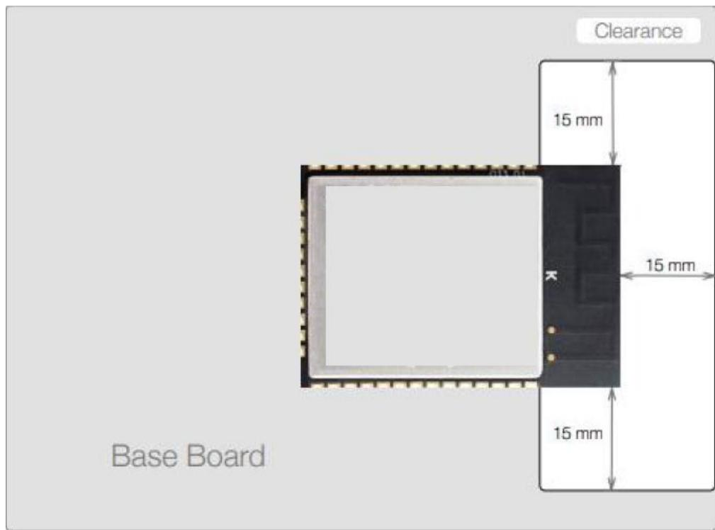
2.2: The side of the IC on the module cannot face the high-frequency components on the drive, but the outside of the drive board;
