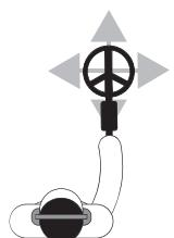
Press the pinpointer button in the app and move the coil horizontally and vertically to find precise location of the target.
