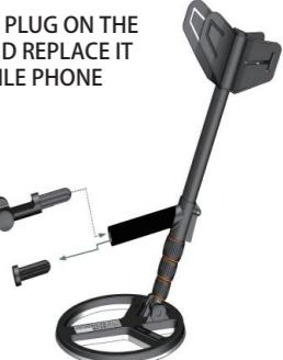
LOOSEN THE NUT ON THE STRUCTURAL ASSEMBLY COUNTERCLOCKWISE, PULL OUT THE TELESCOPIC ROD TO THE RIGHT LENGTH, TIGHTEN THE NUT CLOCKWISE.
