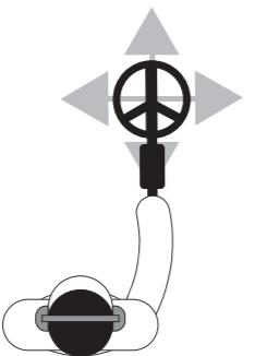
Press the pinpoint button in the app and move the coil horizontally and vertically to find precise location of the target.
