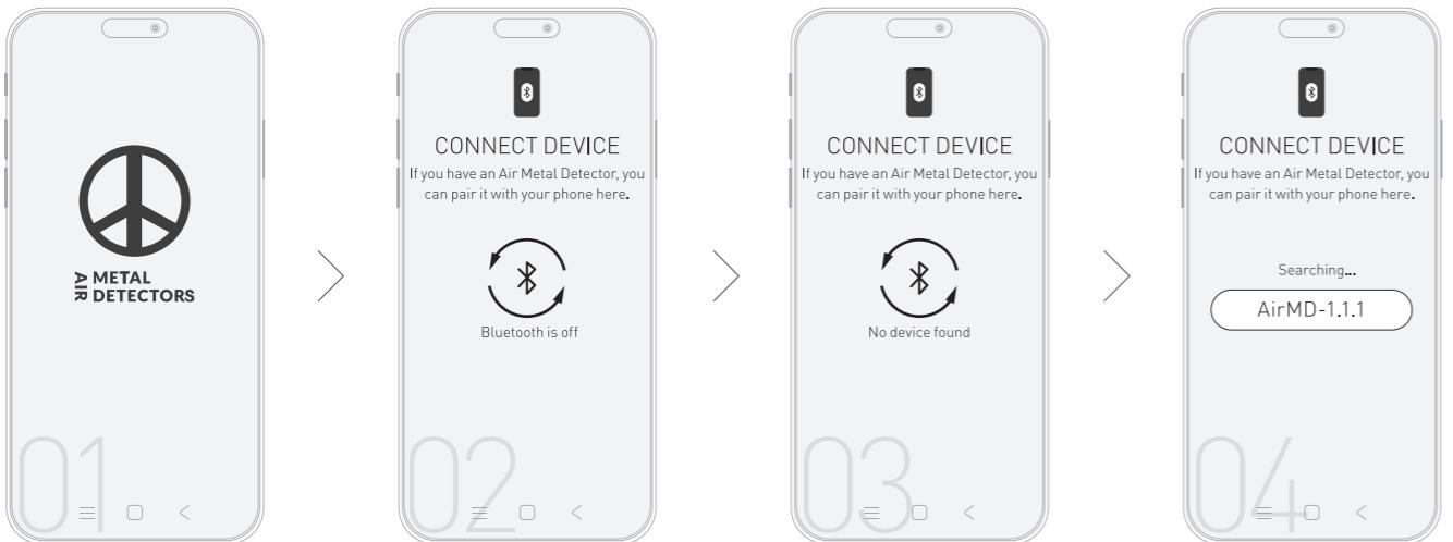
Launch the AIR Metal Detector app and turn on the coil on your AIR MD
