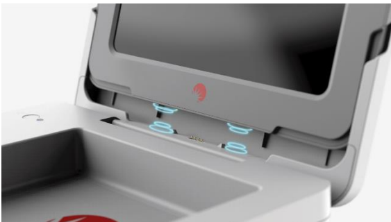
Figure 6: Magnets hold the Tablet in place when it is charging
