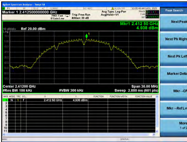
802.11b LOW CHANNEL, CARRIER LEVEL
