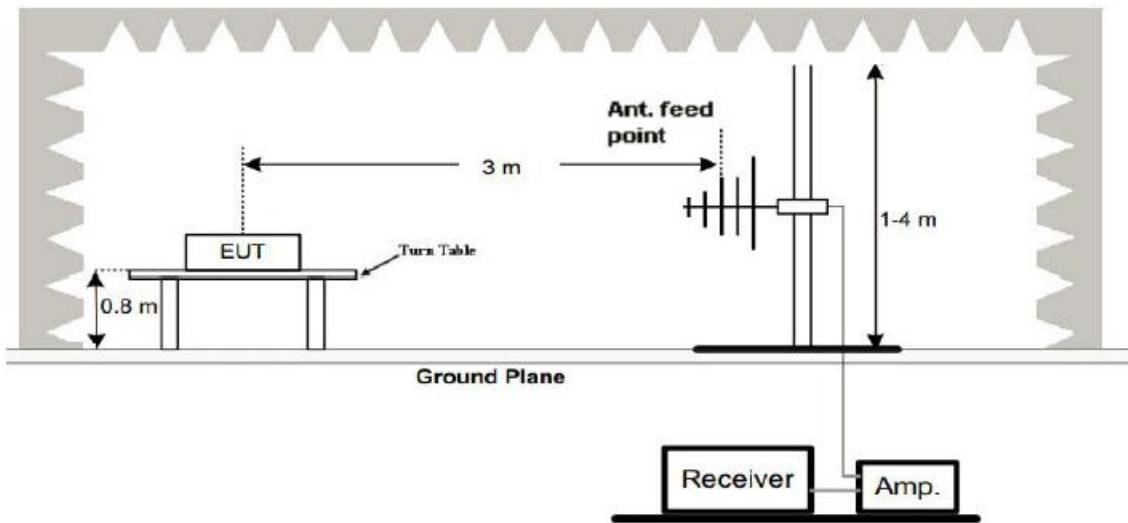
The radiated emission tests were performed in the 3 meters chamber test site, using the setup accordance with the ANSI C63.10-2013. The specification used was the FCC 15.209 and FCC 15.205 limits.
