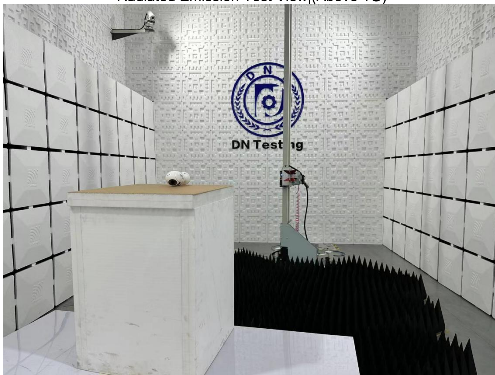
Radiated Emission Test View|(Above 1G)
