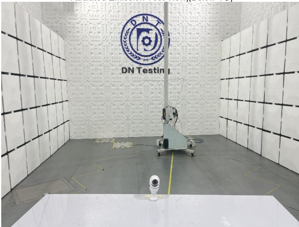
Radiated Emission Test View(Below 1G)
