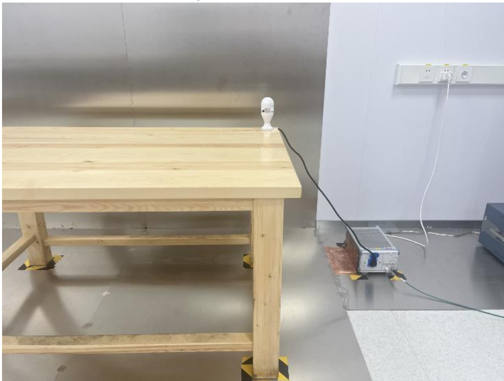
Radiated Emission Test View(Below 1G)
