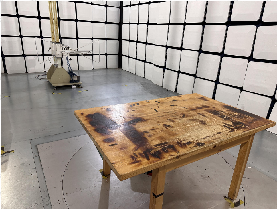
Photo of Radiation Emission Test
