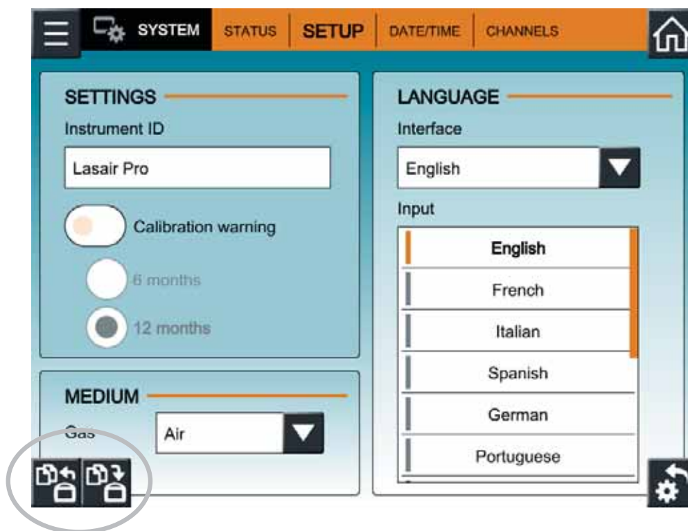
Figure 1-4. Clone Export and Import buttons, SETUP tab, SYSTEM
