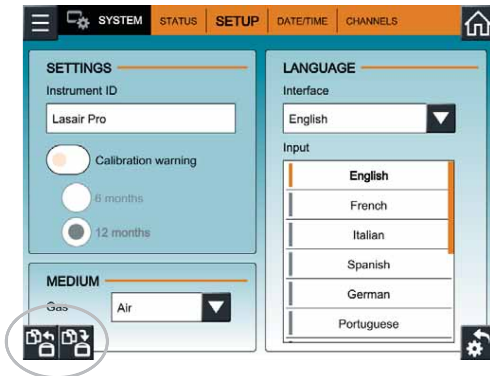
Figure 12-5. Clone Export and Import buttons, SETUP tab, SYSTEM
