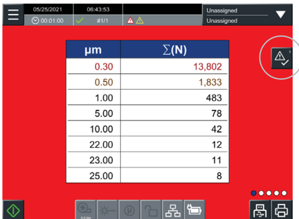
Figure 7-6. Warning/Alarm Acknowledgement button (circled) on the HOME screen
