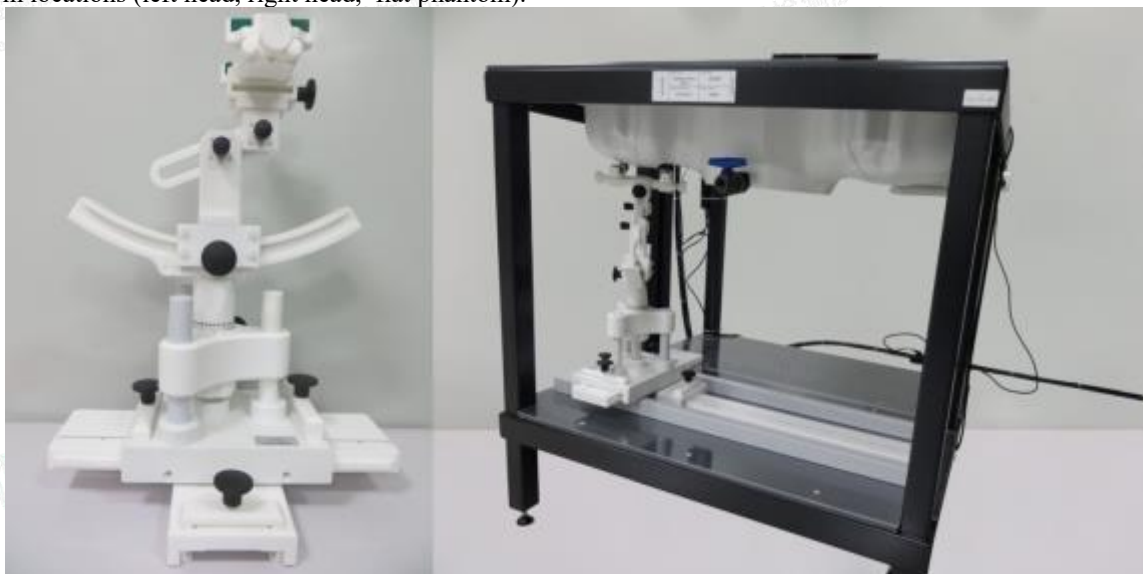
Device holder supplied by SATIMO
