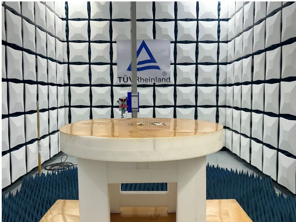
Photograph 4: Set-up photo for Radiated Spurious Emission, above 1GHz (Right earbud)
