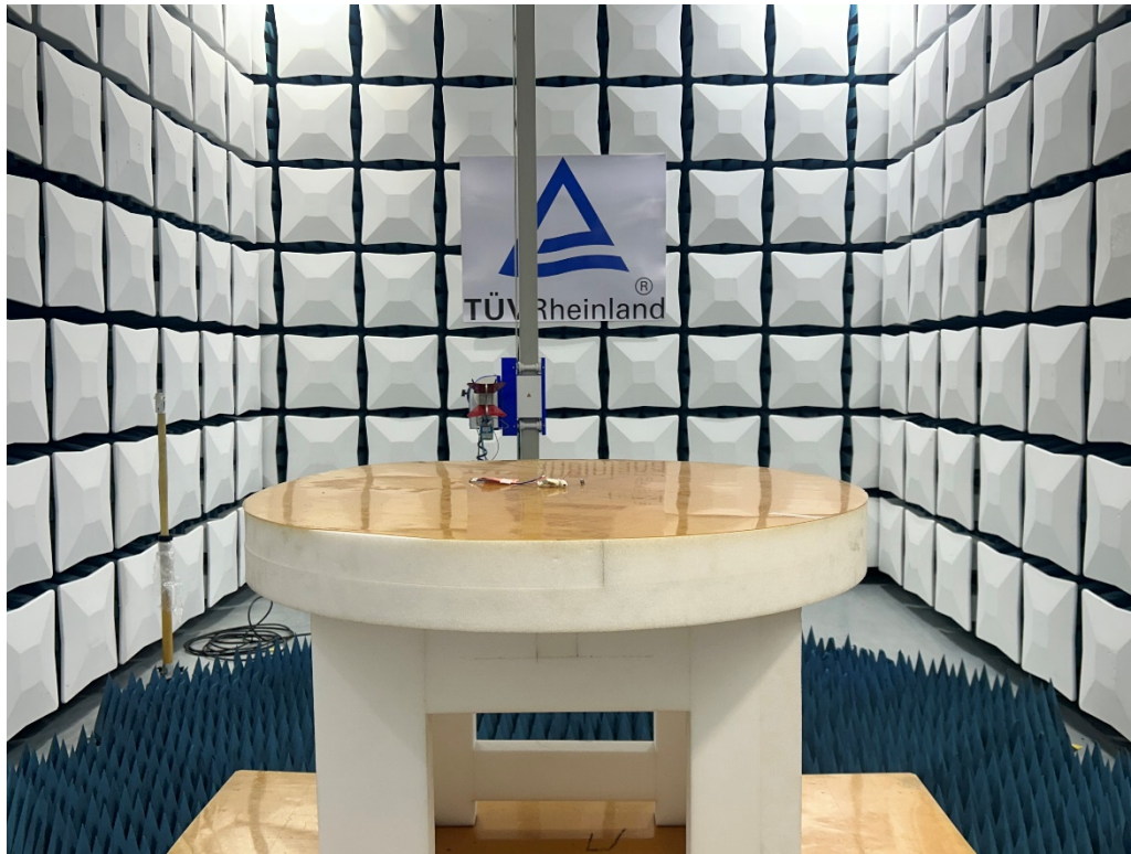
Photograph 3: Set-up photo for Radiated Spurious Emission, above 1GHz (Left earbud)
