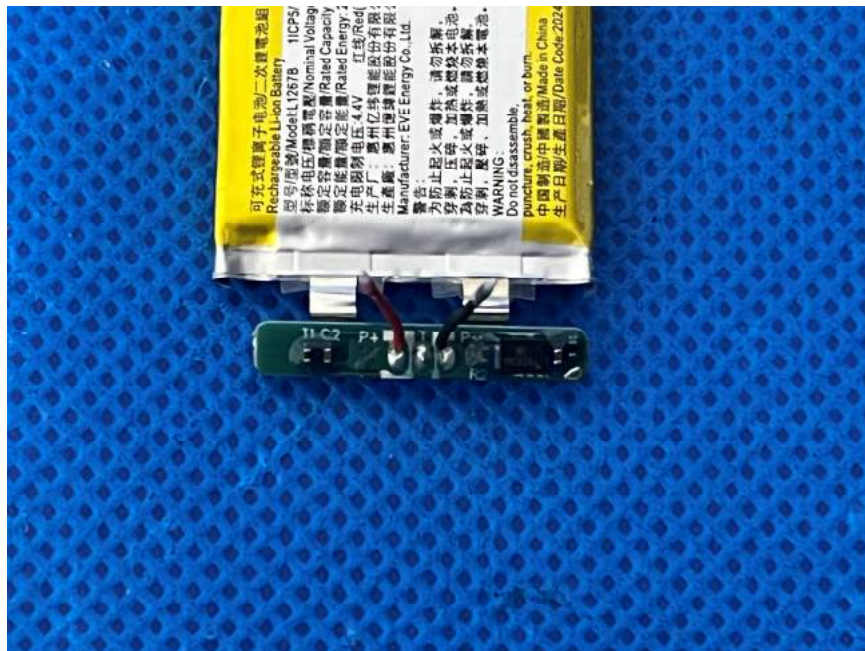
Figure 18: Protective board of charging case battery
