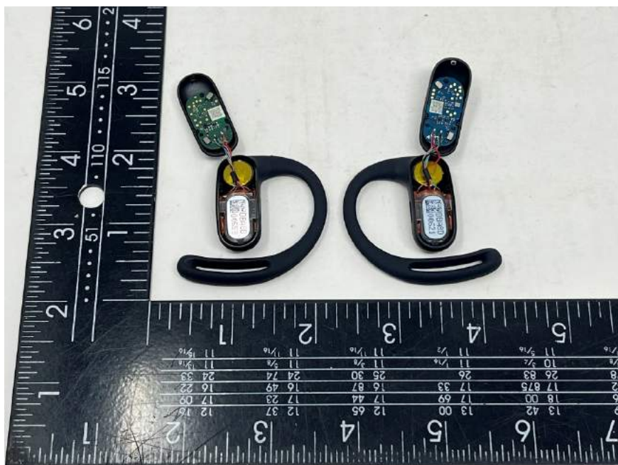
Figure 11: Internal view of earbuds
