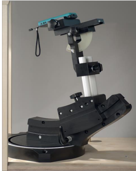
F-2. Device Holder for Transmitters
