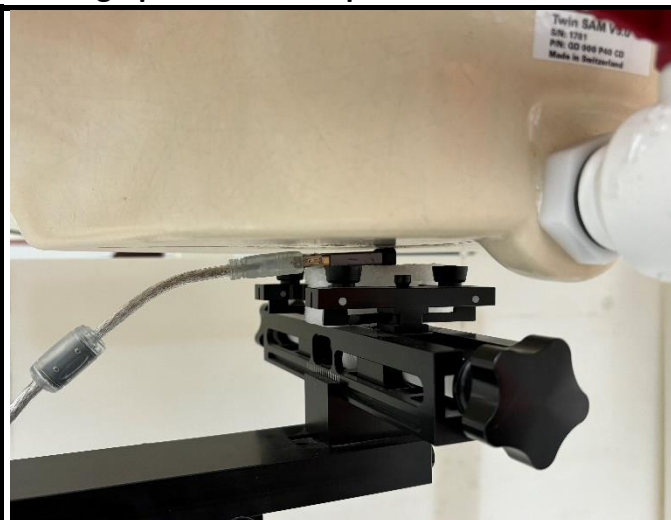
Horizontal-Up of EUT with 0 cm Gap
