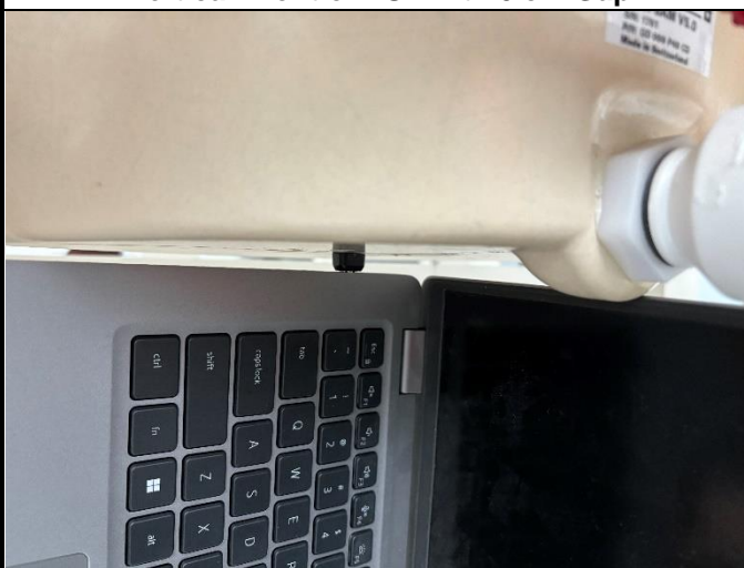
Tip Mode of EUT with 0 cm Gap
