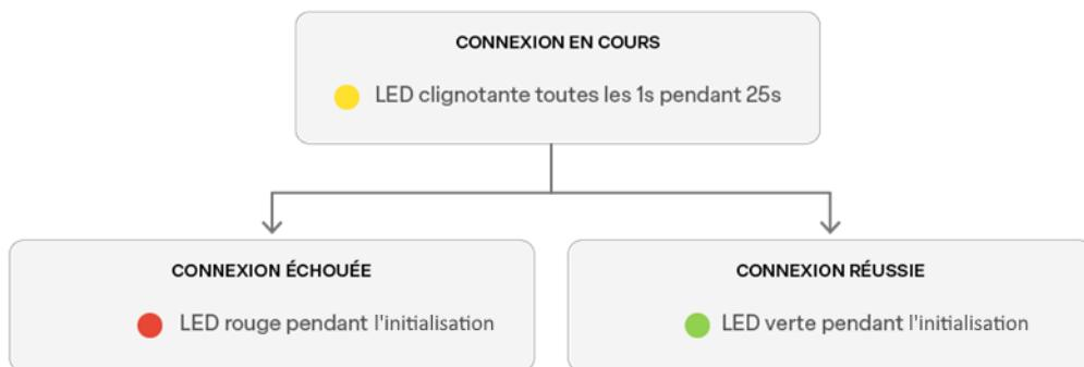
At the end of the connection phase (approx. 25 seconds), the product is ready for use. In the event of failure, the product will immediately attempt a second connection to the network, and then periodically (more information is available in section 0
