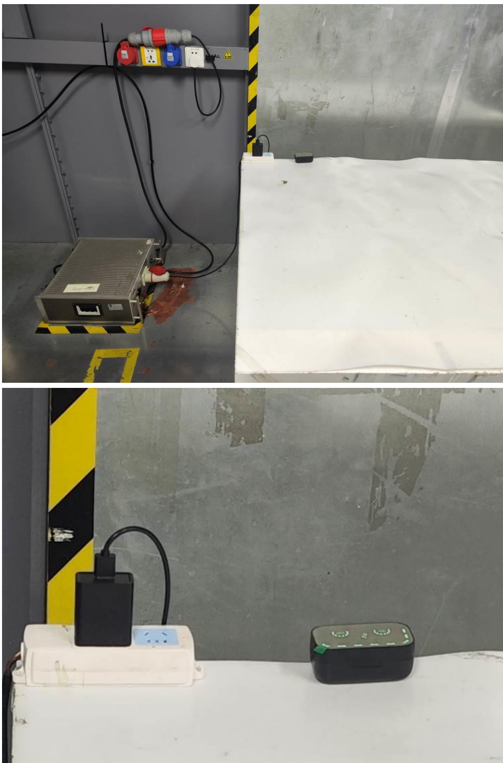
Photo of Conducted Emission test
