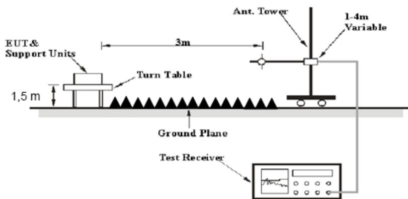
The radiated emissions were performed in the 3 meters distance, using the setup accordance with the ANSI C63.10-2013. The specification used was the FCC 15.205, 15.209, and FCC 15.231 limits.
