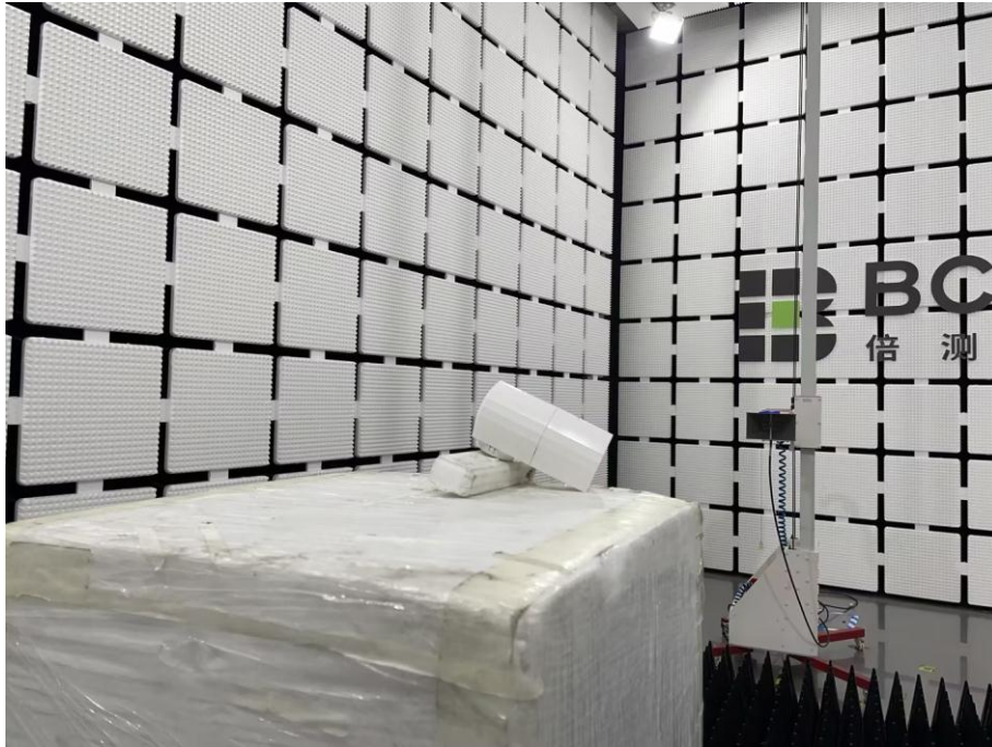
Spurious Emission Test Setup (Above 1GHz)
