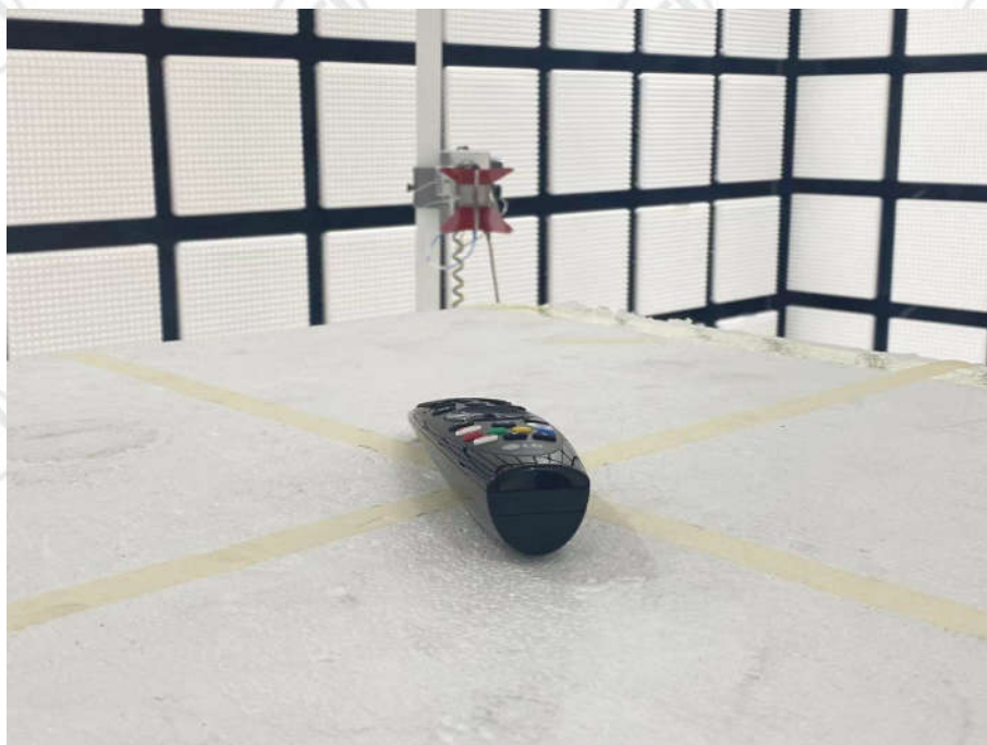
Radiated spurious emission Test Setup-3(Above 1GHz)
