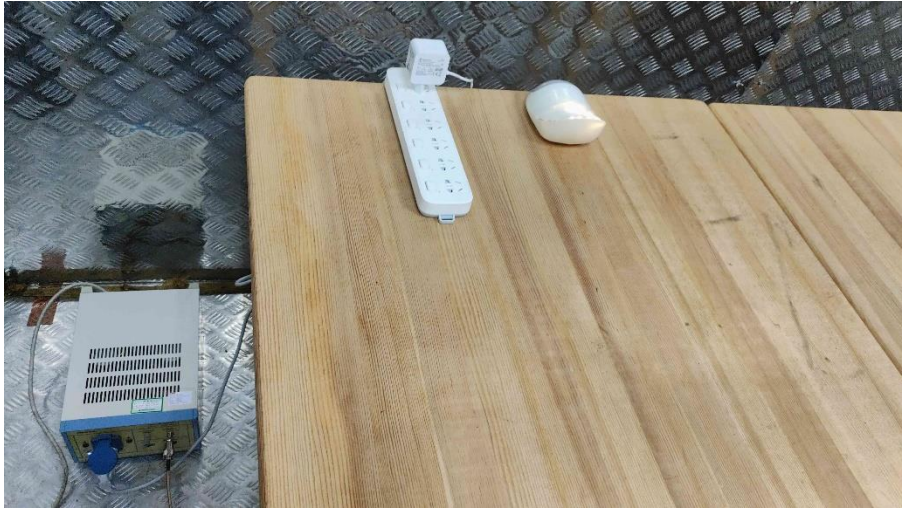
Conducted Emission test view_AC
