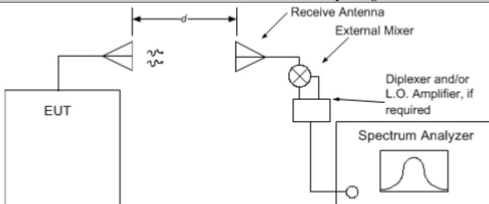
The following procedure shall be used for measurement of the bandwidth for millimeter-wave devices:
