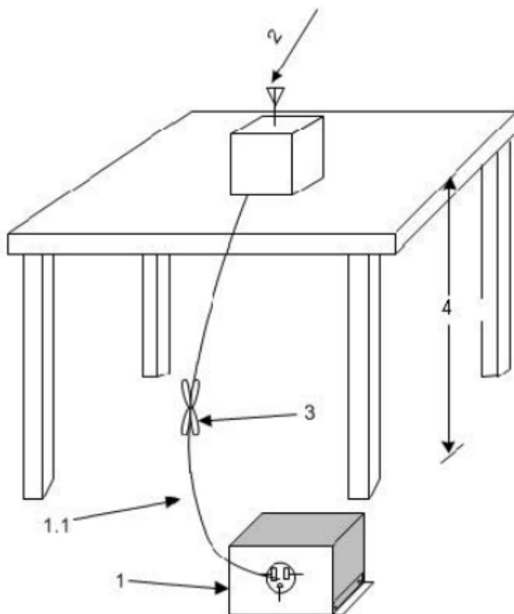
1—A LISN is optional for radiated measurements between 30 MHz and 1000 MHz but not allowed for measurements below 30 MHz and above 1000 MHz. If used, then connect EUT to one LISN. Unused LISN measuring port connectors shall be terminated in  $50\ \Omega$  loads. The LISN may be placed on top of, or immediately beneath, the reference ground plane.
