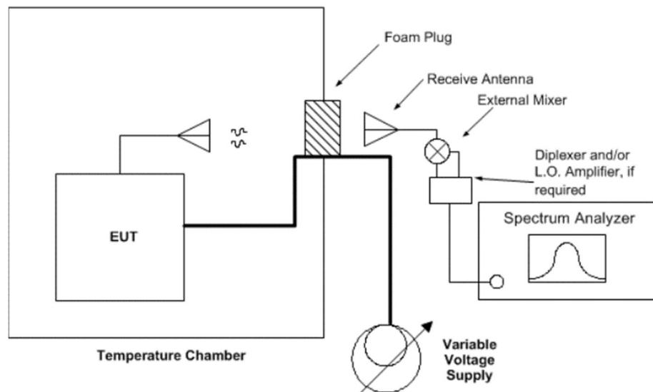
The following procedure shall be used for determining frequency stability of millimeter-wave systems:
