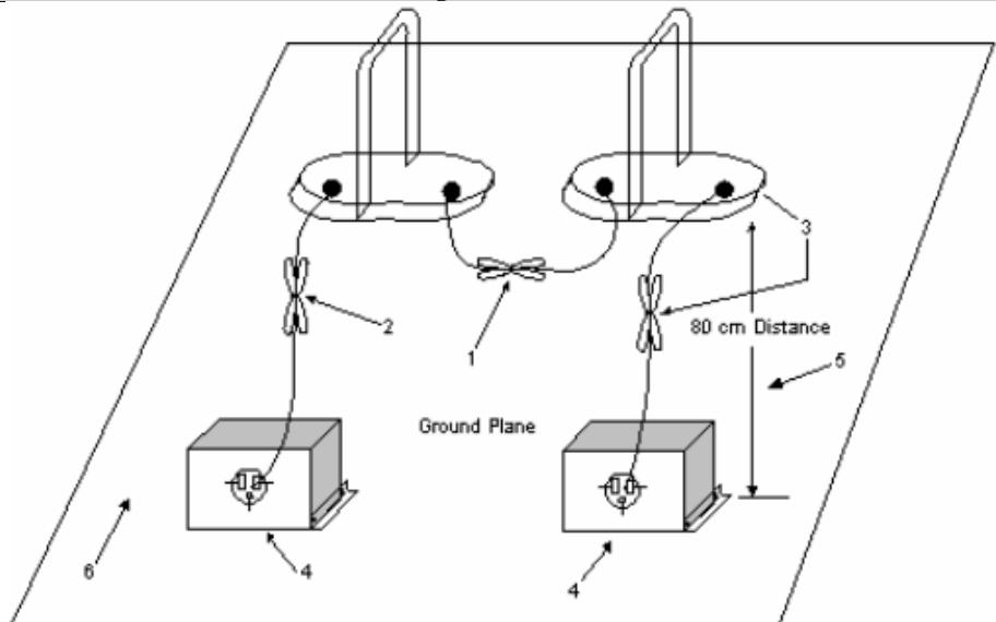
1—Excess I/O cables shall be bundled in the center. If bundling is not possible, then the cables shall be arranged in serpentine fashion. Bundling shall not exceed 40 cm in length.
