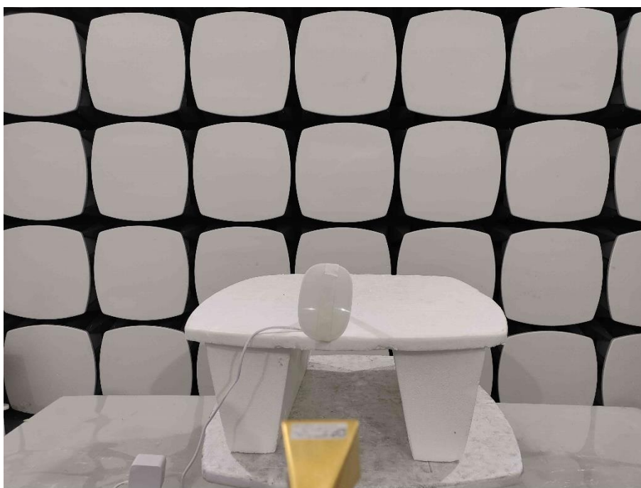
Radiated Emission test view (Frequency from 60GHz to 90GHz)
