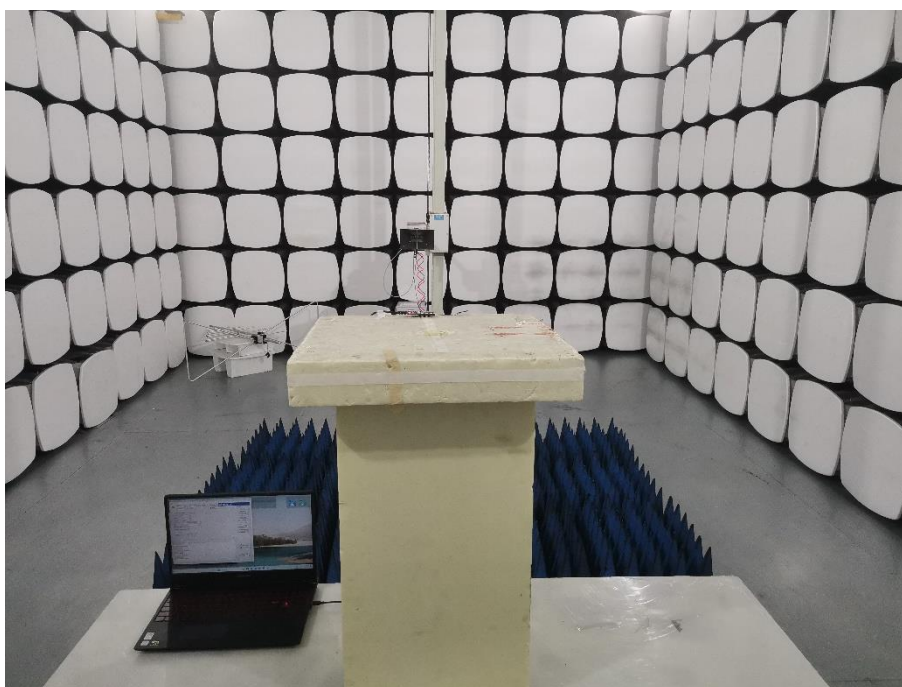
Radiated Emission test view (Frequency above 1GHz)
