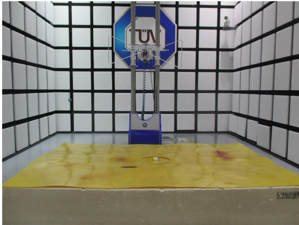
Radiated Emission Test below 1GHz
