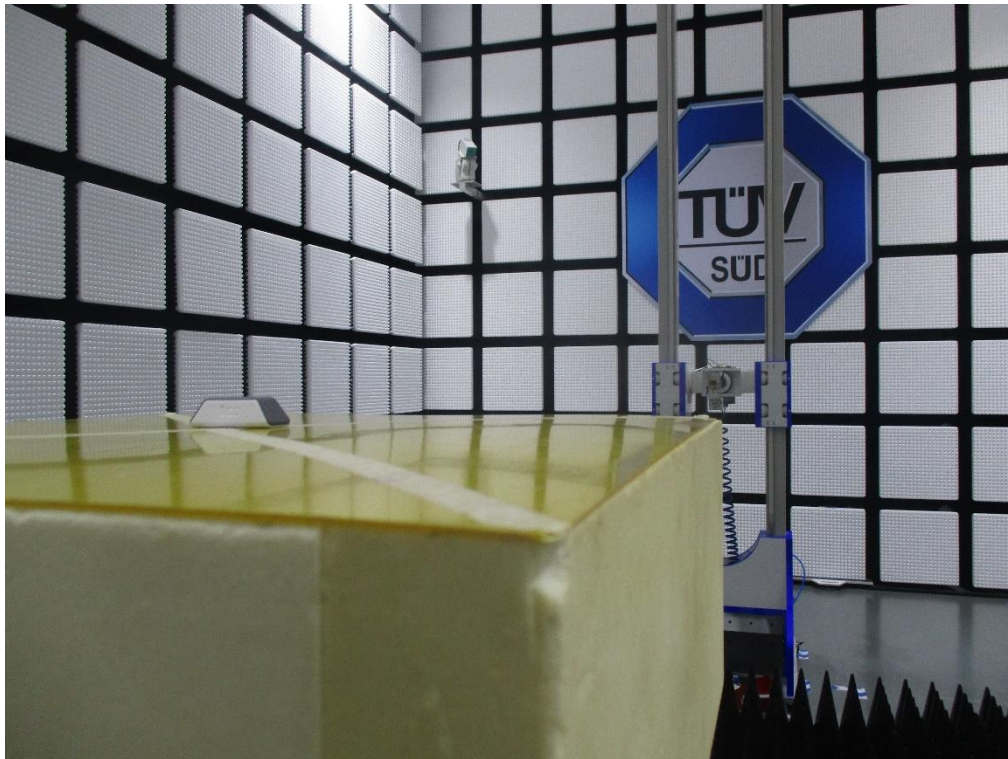
Radiated Emission Test above 18GHz
