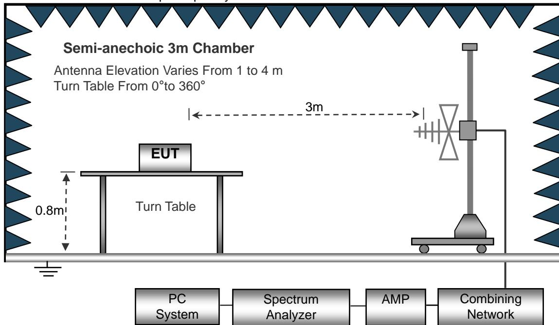
(C) Radiated Emission Test-Up Frequency Above 1GHz
