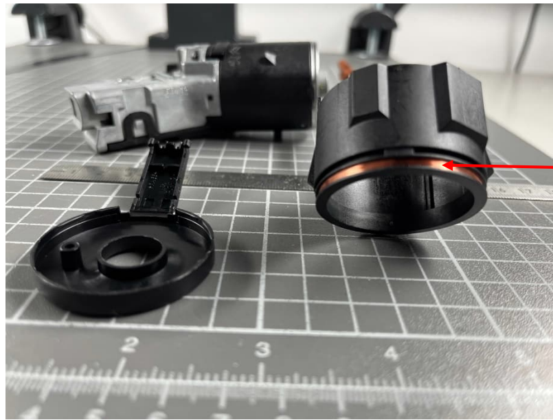
Ignition lock, 125 kHz loop antenna position
