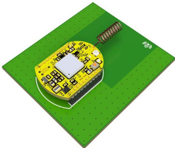
Use copper pour ground planes on the top and bottom layers; use multiple GND net via holes to tie separate ground plane areas tightly together.
