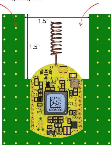
Sockets can be used on the host circuit board for ease of removing and replacing WillowBee. Alternatively, WillowBee can be soldered directly to the host circuit board.
