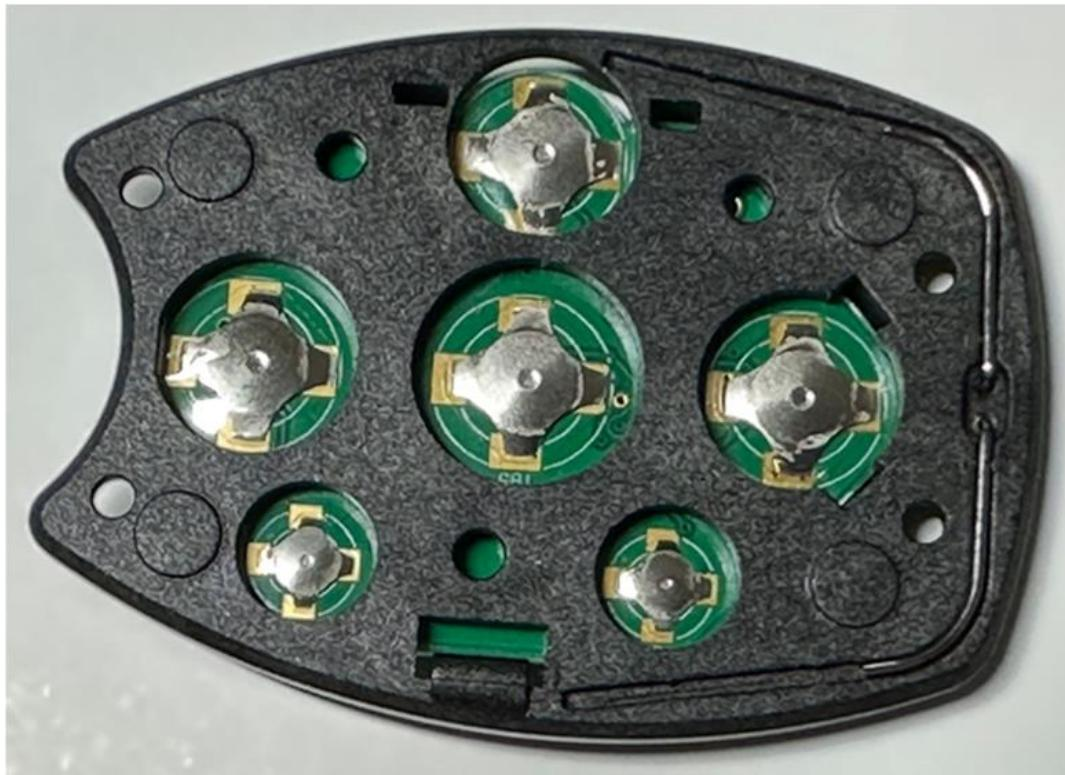
The antenna is a custom dipole, fabricated as an integral part of the internal housing. It cannot be changed or replaced, since it is integrated into the housing. The antenna gain is approximately -3dB.
