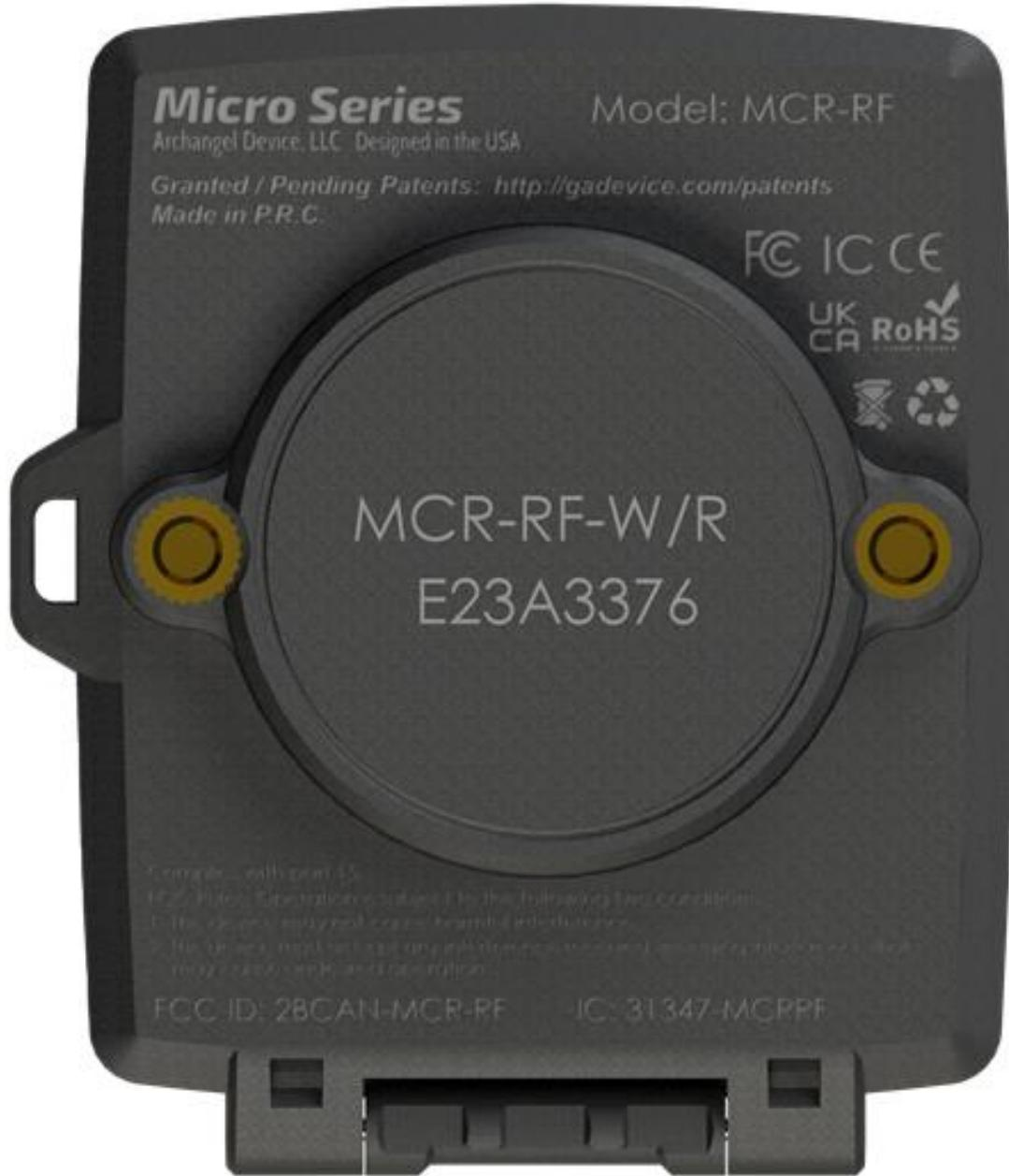
The FCC/ISED label will be etched onto the plastic case of the EUT. The label area measures 1.5" wide by 1.75" tall.
