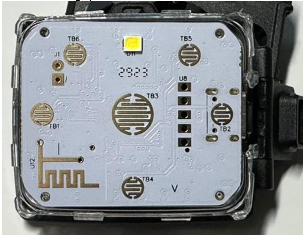
Photograph of PC Board: Foil Side with Antenna
