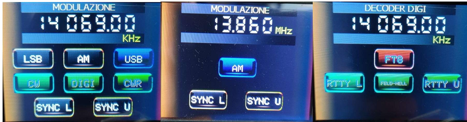
Screen for selecting the modes/types of modulation used for the HAM ranges only (amateur ranges) and the SW range, and with the frequency used at the top
