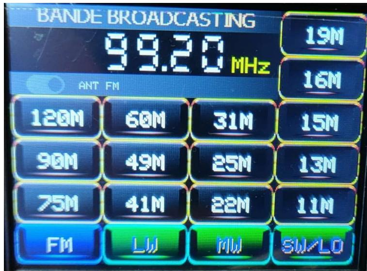
Screen of choosing the broadcasting band to use , with an indication at the top of the frequency in current use.
