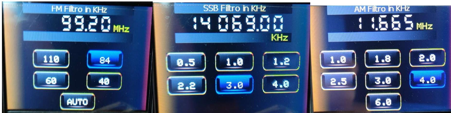
Bandwidth selection screens to use, for FM / AM / SSB, with indication at the top of the frequency and mode in current use.
