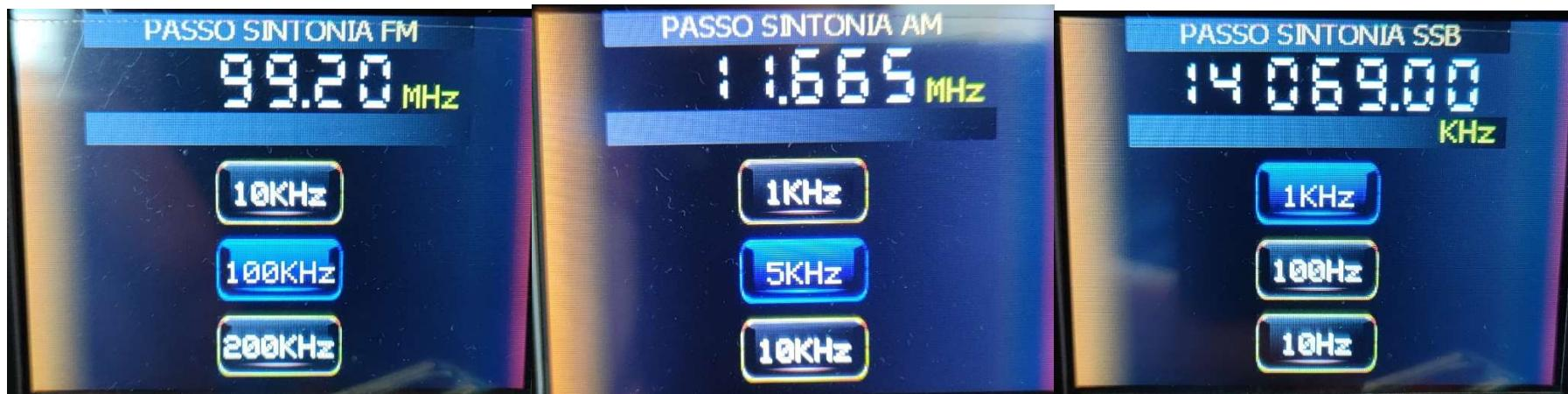
Screens for choosing the STEP tuning pitch to be used for the FM - AM - SSB bands, with indication at the top of the current frequency.
