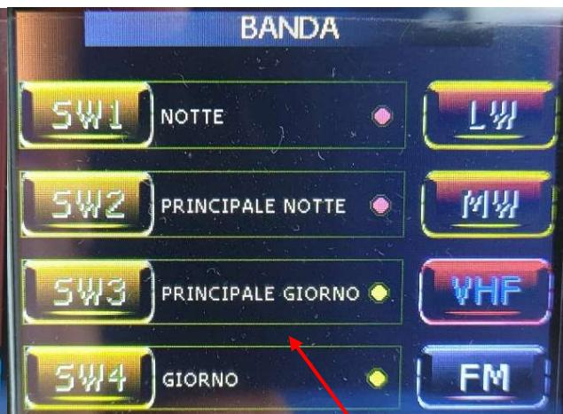
Band selection page displayed in RETRO mode, with buttons for retro bands and color indication of wave propagation conditions in relation to real-time conditions with data obtained via WiFi
