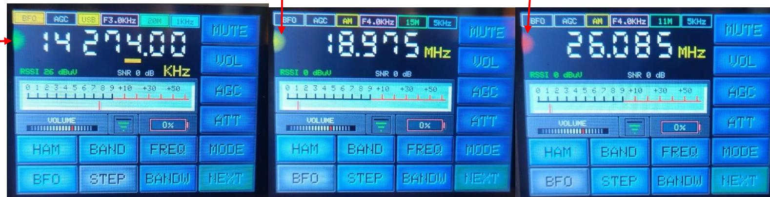
Reception in the HF bands with color indication of the conditions of propagation of radio waves in the range used:
