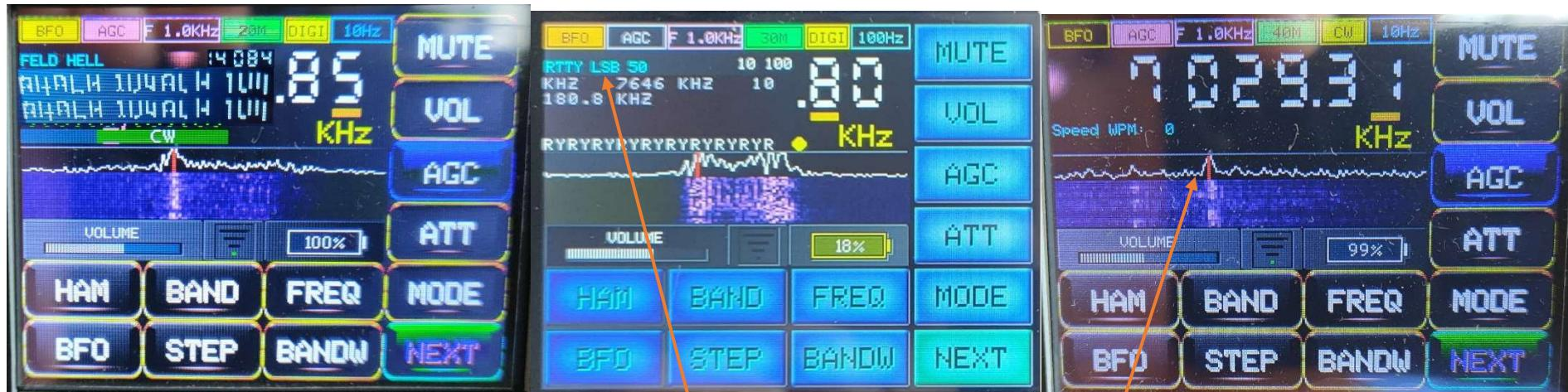
Decoding screen of the FELDHELL digital mode (also called "Minifax"). To center the writing long press on the display receiving messages, the writing will change to yellow, then use the encoder to adjust; press again to return.
