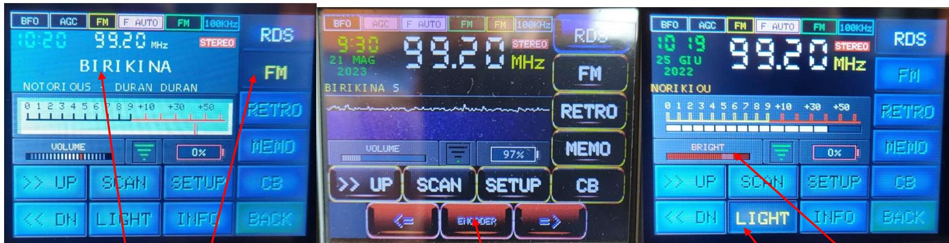
Screen appearance with FM button enabled. You can switch the encoder to the FM stations of the band stored in the memory bank for the current city.
