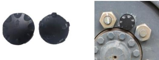
Separate the sensor base, mix AB glue in a 1:1 ratio, and place an appropriate amount on the base. First, stick the base to the selected installation position on the wheel; After the glue solidifies, install the sensor, or use a bracket to assist in installation.
